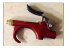
Correct (nozzles with relief holes, or star-tipped)
