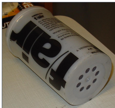
Figure 2: An f/air canister with exhaust ports on the bottom
