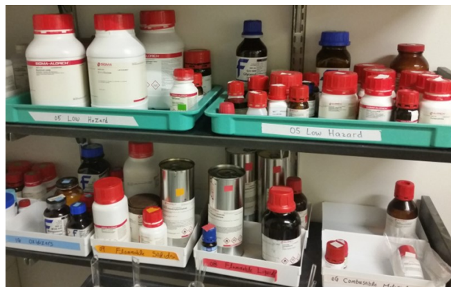
Figure 1: Storage bins used to segregate different hazard classes
