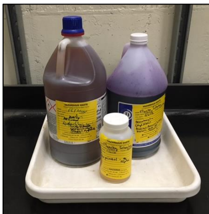
Figure 3.3 – Example of Secondary Containment
